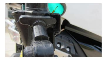
Note: The charging handle guard area is extra long and may need to be trimmed-back based on the size of the charging handle – otherwise the weapon may be scratched when installing or removing from mount. Trim with a cordless hacksaw, sand and then touch-up with black paint.
